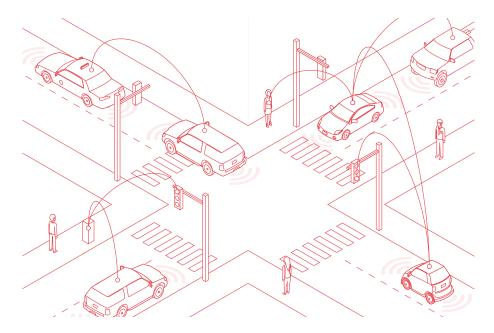
This type of innovation could, in the future, create wider connected infrastructure to which vehicles can connect, allowing them to join a vehicle platooning service operated by specialized traffic management centers or purpose-built Al<sup>24</sup>. This connectivity, called vehicle-to-everything (V2X), combines V2V and V2I, and is enabled by the multitude of communication systems and sensors that are now common in modern connected vehicles.
