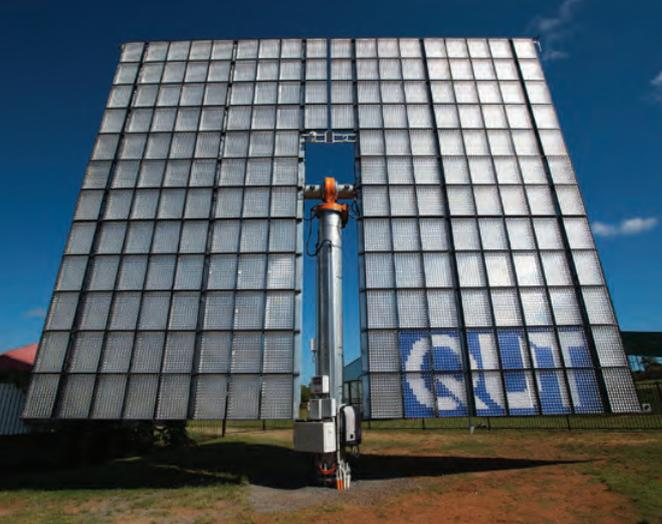
A concentrated photovoltaic (CPV) system being tested in a joint QUT and Sumitomo Electric Industries project at the Queensland Government's Redlands Research Facility.
