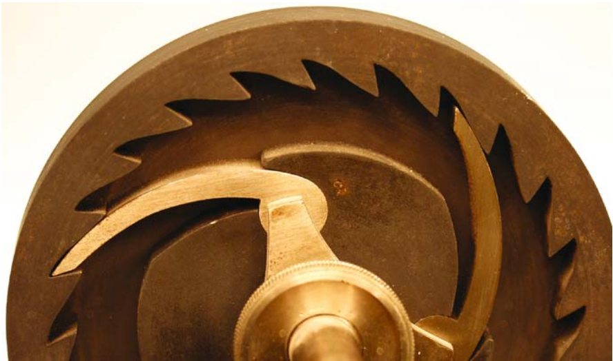
Color Plate 4. Close-up of ratchet-wheel coupling. Reuleaux–Voigt Model N-7, Cornell University Collection of Kinematic Models, nickel-plated brass and cast iron, Berlin, circa 1882 (Photo, F.C. Moon)
