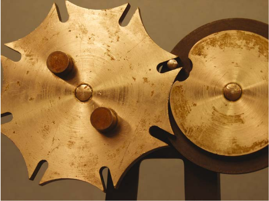
Color Plate 3. Geneva-wheel intermittent mechanism for watches. Reuleaux–Voigt Model N-8, Cornell University Collection of Kinematic Models, nickel-plated brass and cast iron, Berlin, circa 1882 (Photo, F.C. Moon)
