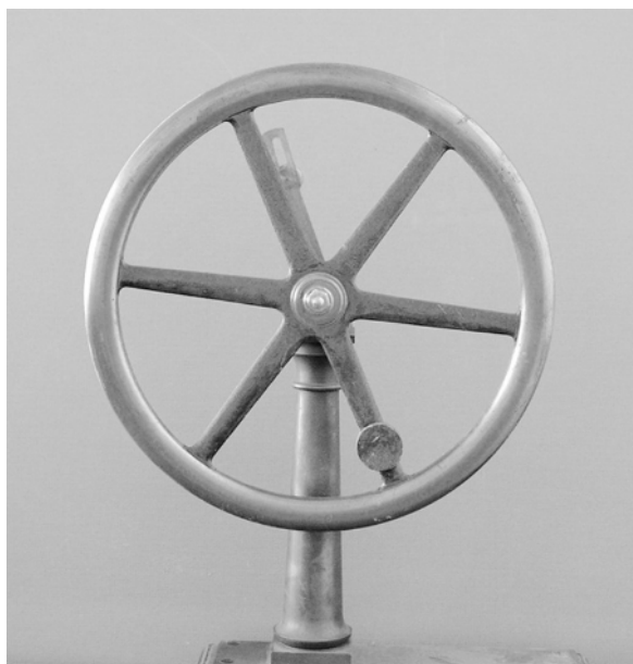
Figure III.20b. Flywheel or balance wheel: Reuleaux-Voigt Catalog, Model N-27 (Cornell Collection of Kinematic Mechanisms)
