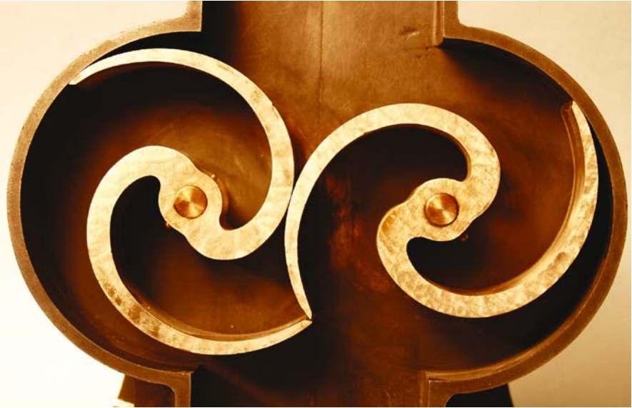
Color Plate 7. Spiral positive-displacement pump. Reuleaux–Voigt Model I-4, Cornell University Collection of Kinematic Models, nickel-plated brass and cast iron, Berlin, circa 1882 (Photo, F.C. Moon)
