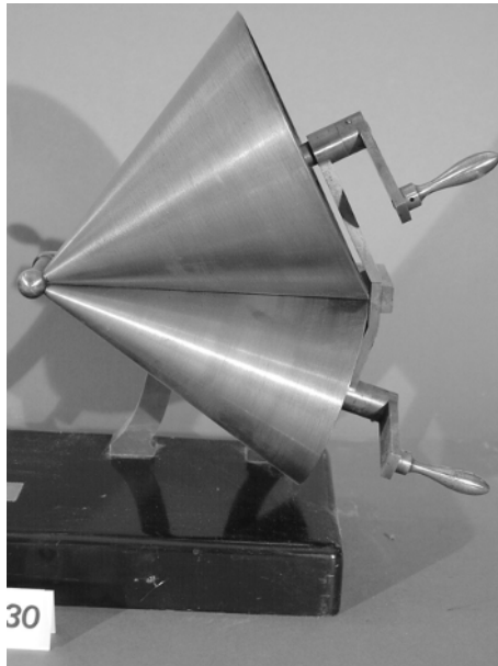
Figure III.16b. Conical friction wheels: Reuleaux Model, Deutsches Museum (c. 1880)
