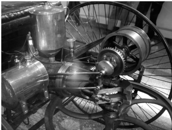
Figure I.13. First automobile of Carl Benz and the list of basic machine elements and mechanisms (c. 1885) (Courtesy of the Deutsches Museum, Munich)
