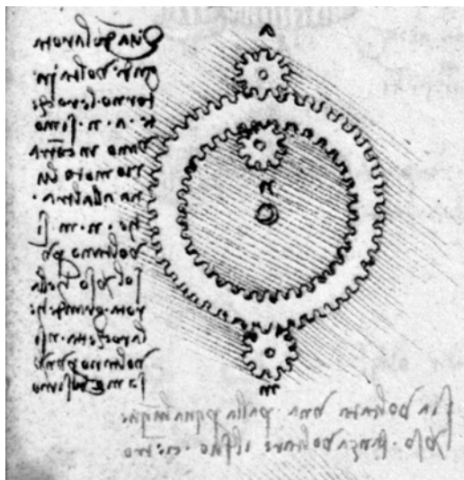
Figure III.15a. Planetary-epicyclic gear train: Codex Madrid I , Folio 13v
