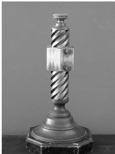
Figure III.7b. Screw pair: Reuleaux–Voigt Catalog, Model A-1 (Cornell Collection of Kinematic Mechanisms)
