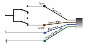
When first connected to power the motor will run a full cycle to set the end limits
