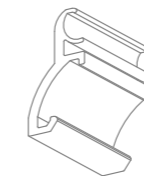
COVER HINGE to hold cover plate, installed on either side
