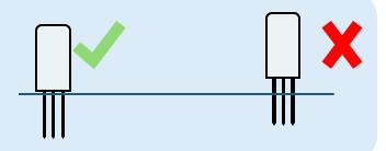
Place the pins perpendicular to the substrate
