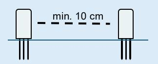
Place the pins all the way in the substrate
