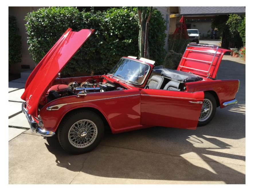
The 2,1388cc inline-four sends power to the rear wheels through a four-speed manual gearbox featuring a Laycock de Normanville overdrive. In 2000 the clutch master cylinder was replaced. Many additional photos of the car can be viewed in the gallery below.
