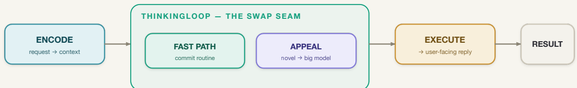
Figure 42. The runtime lifecycle of a single turn. The ThinkingLoop is the one seam where “how to decide” plugs in; the safety gate sits underneath it, armed from boot.
