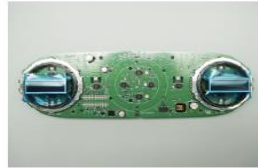
Full Automatic Temperature Control System
