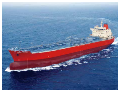
Product tanker for refined petroleum products such as diesel oil, naphtha, and gasoline
