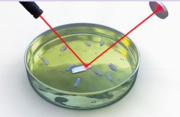
In 2020, McKendry improved upon a proposed mechanical cantilever-based sensor which is capable of detecting AMR within ~45 minutes. It was demonstrated to be effective both in lab conditions and with clinical strains of AMR *E. coli*.
