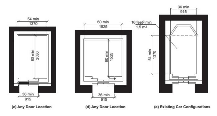
FIGURE 3 Excerpt of FIGURE 407.4.1 of ICC A117.1-2009 Inside Dimensions of Elevator Cars
