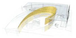
The cellular wall is one of the most captivating elements in the SNHM design. Besides its architectural appearance it also has an important function in the structural system to distribute both horizontal and vertical forces. It requires large efforts to create the optimal configuration that meets both its architectural and structural objectives. This includes the structural material of the cellular wall.
