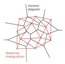
Fig.3.7 Voronoi diagram and the associated Delaunay triangulation [Source: Architectural Geometry]
