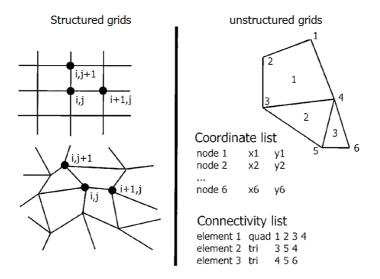
Fig. 3.4 The logic of structured and unstructured grids [Gable, 1996]
