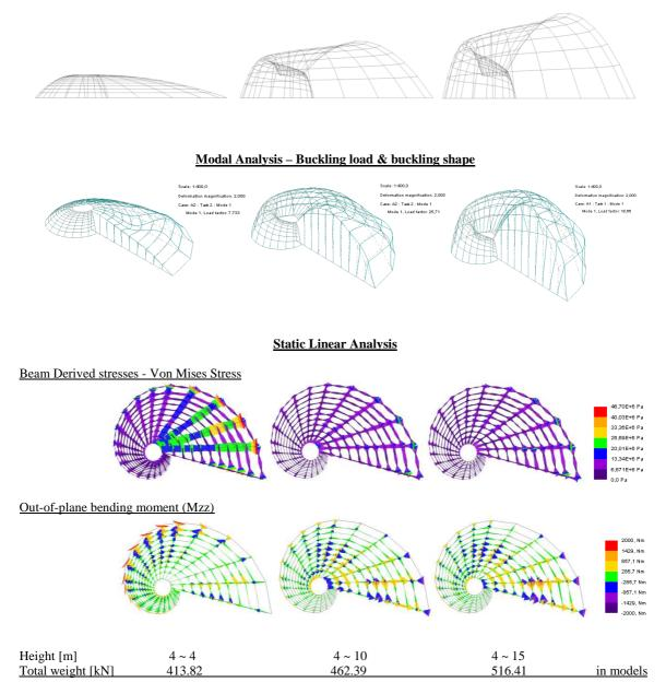
With the parametric model, the ratio of height-span can be explored to build up a good structural form;
