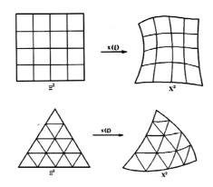
Fig.3.5 Boundary-conforming quadrangular & triangular grid [Liseikin, 1999]
