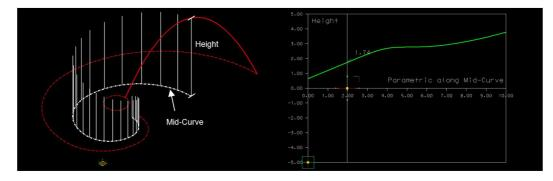
Fig.4.8 Parabola thrust line defined by Mid-Curve and predetermined Height (Left); Law-Curve (Right)
