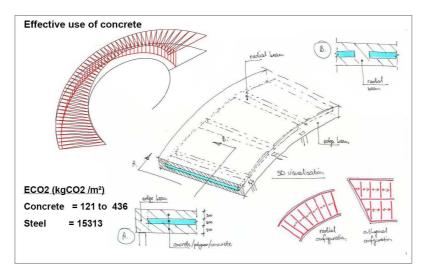
Fig 2.3 Ramp and roof structure
