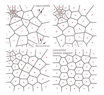
Fig.3.8 Steps of Centralized Voronoi Diagram [Source: Architectural Geometry]
