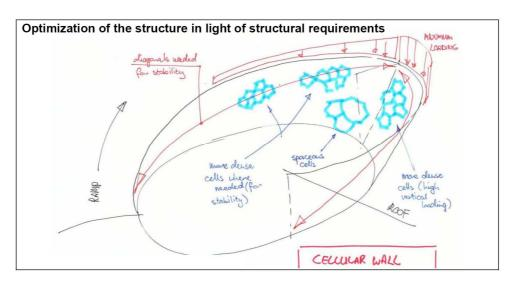
Fig 2.7 Structural principles of cellular wall configuration
