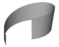
The surface of the cellular wall (of SNHM) can be defined as **Single curved surface (developable)**, which is curved in only one direction (one of the principal curvatures is zero) and can therefore be unrolled to a plane.
