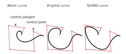
Fig.3.2 three types of free form curves used in design [Source: Architectural Geometry]
