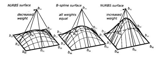
Fig. 3.3 weights as shape parameters of NURBS surfaces : increasing a weight pulls the surface towards the corresponding control point, decreasing a weight shows a push-away effect [Source: Architectural Geometry]
