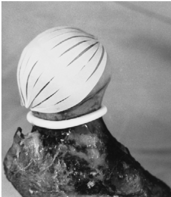
FIG. 1. Femoral head with Fuji pressure-sensitive film.
