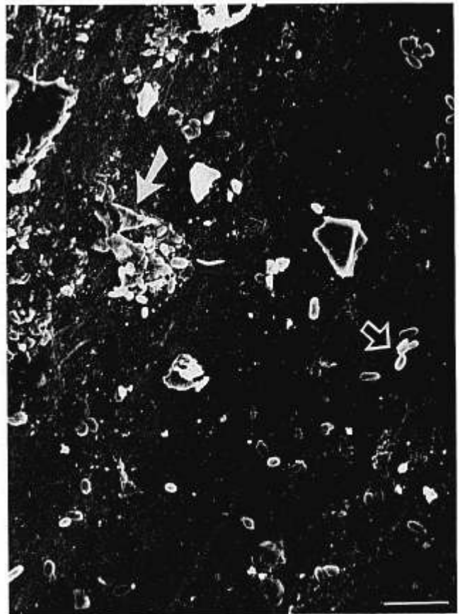
Figure 3. Scanning electron micrograph of stainless steel exposed to Mycobacterium tuberculosis (clinical strain). There are few adherent rod-shaped organisms (white and black arrow) and thin biofilm (white arrow) adherent on the surface of the stainless steel. Bar = 5 \mu m
