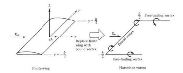
Placing an infinite number of these horseshoe vortices over a wing allow us to find the lift distribution. The reason why this is needed is explained in detail in Anderson, but a somewhat intuitive motivation to why a single horseshoe vortex doesn't suffice when it comes to modelling the lift distribution is the fact that the downwash in the trailing vortices would be infinite in magnitude (again, see Anderson).
