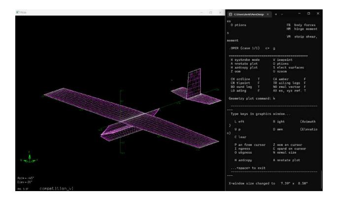
If you enter the geometry plot window by, say, clicking on it, you can hit the keys "L," "R," "U," and "D" to move the plot around. You can also pan around with "P," zoom with "Z," and do some other cool things as the AVL terminal shows. Play around with these for a bit, and get used to interpreting what each key means by what AVL tells you there.
