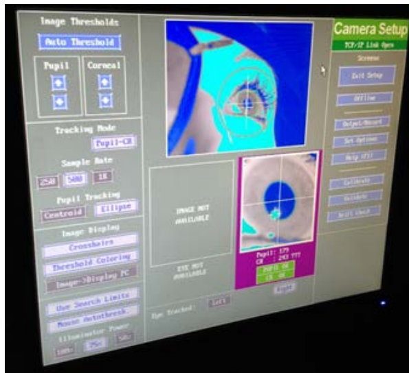
Figure 13. An example of the “Camera Setup” screen on the host computer. Here, the eye is set up such that there are good pupil and corneal reflection thresholds.
