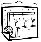
This configuration will work with one 3V battery. The battery will drain faster the more LEDs you add in parallel.
