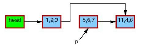
Please note that readers are not permitted to maintain references to element 5,6,7 after exiting from their RCU read-side critical sections. Therefore, once the <code>synchronize\_rcu()</code> on line 4 completes, so that all pre-existing readers are guaranteed to have completed, there can be no more readers referencing this element, as indicated by its black border below. We are thus back to a single version of the list.
