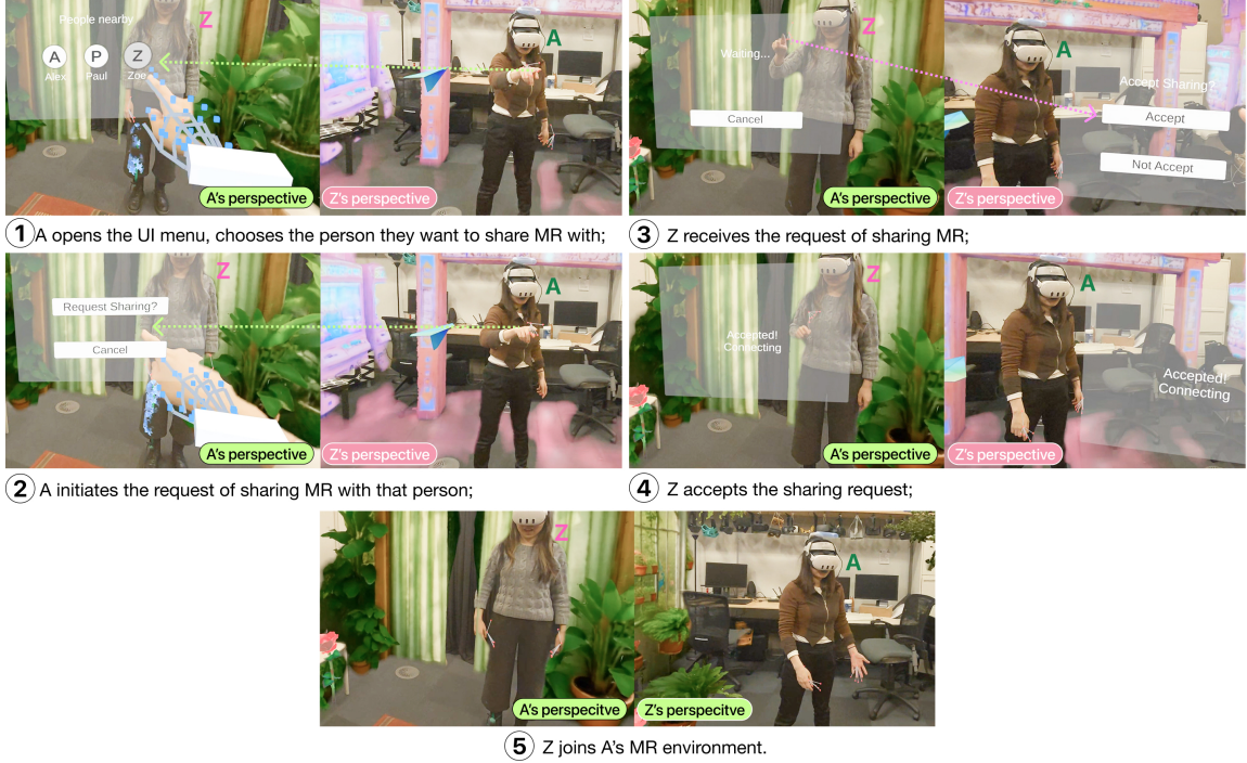
Fig. 2. The MenuPort UI-menu sharing flow. (1) A opens the menu and selects Z; (2) A sends the sharing request; (3) Z receives the request; (4) Z accepts; (5) Z joins A's MR environment. Each step shows both participants' perspectives.
